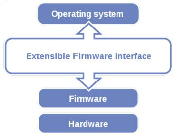
Figure 5-1. Extensible Firmware Interface Diagram
